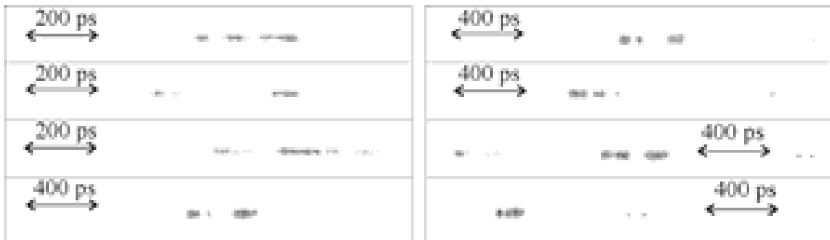
Fig. 4.3.2 Several streak camera measurements of the frequency doubled output signal from the mode-locked \text{Yb}^{3+} -fiber laser.
