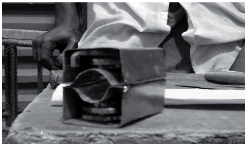
Fig. 2: Construction of the water ionizer showing the magnet, the Yoke, and the reflector.
