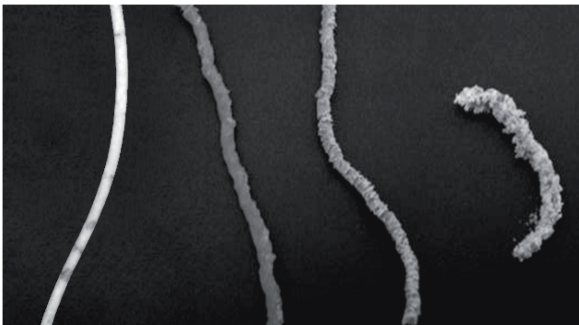
Figure 3.14: Strands of formulation FF-K (FF+PVA-AA-MMA = 1+3 weighted parts) extruded at process temperatures 90, 120, 150 and 180 °C (from left to right)
