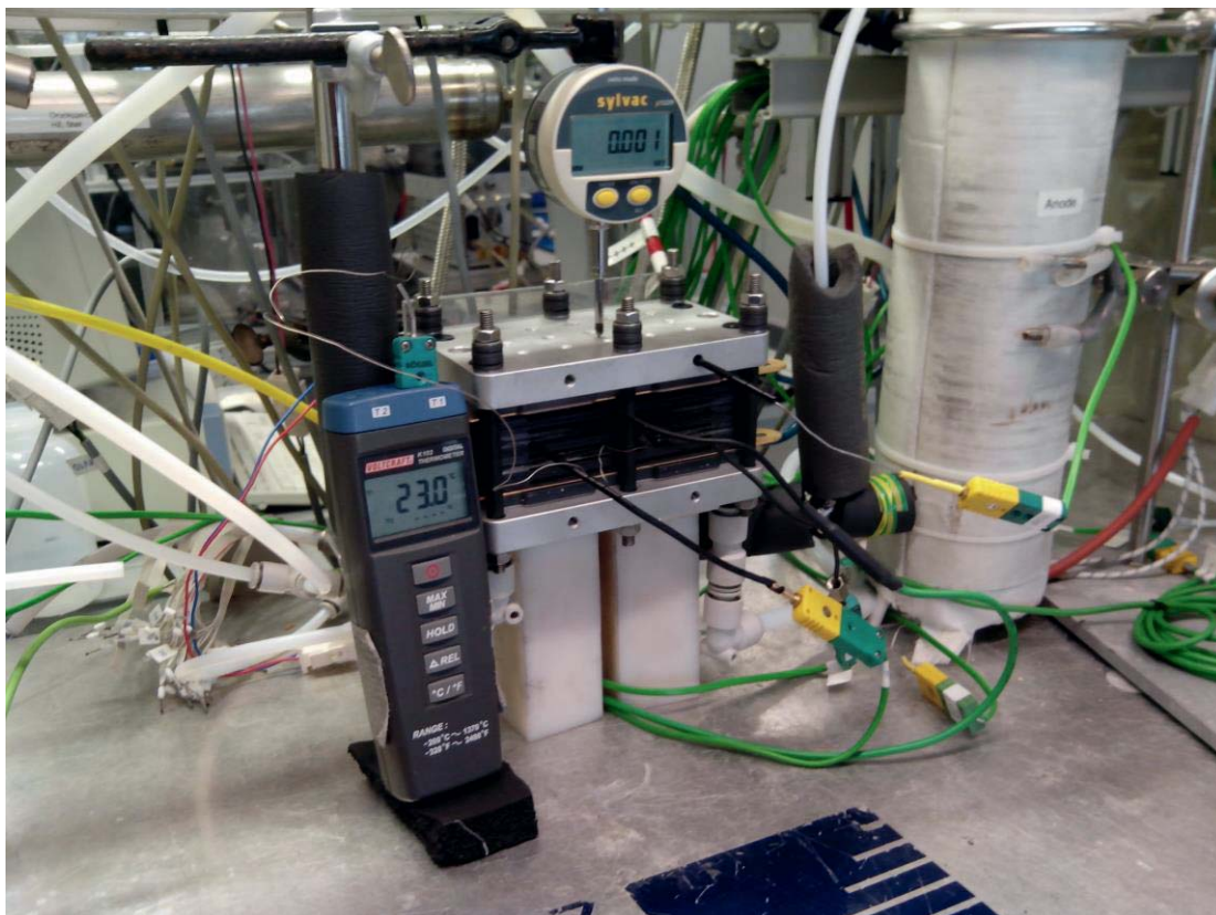
Figure 3.2 Experimental set-up for the thermal expansion measurements
