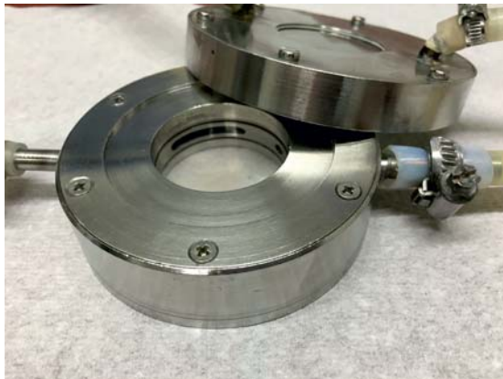
Figure 4.16: Vessel and lid (microscope cell) with static inner volume, heat exchanger temperature controlled by thermostat
