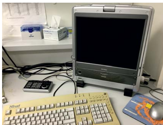
Figure 4.19: Keyence VHX 500F control unit with screen
