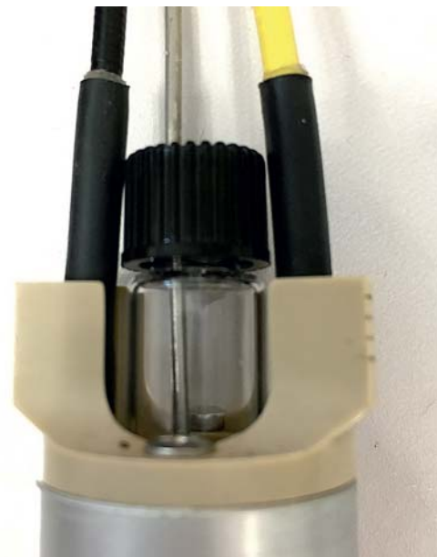
Figure 4.2: Image of turbidity measurement insert for HPLC tubes
