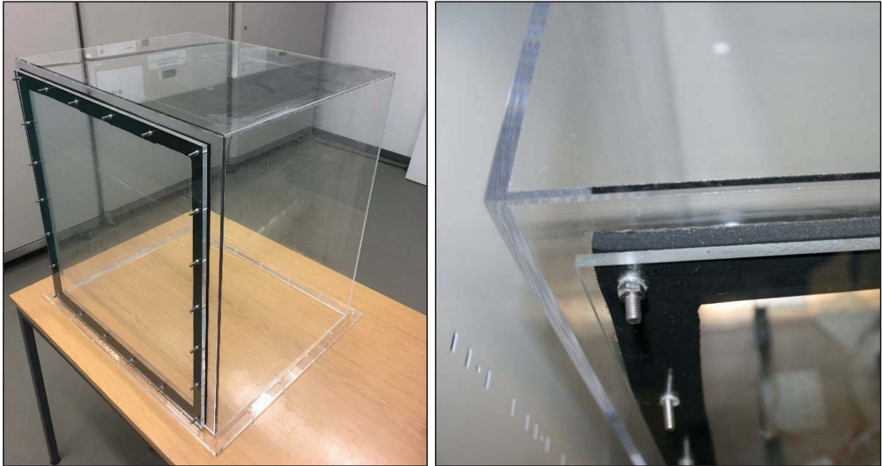
Fig. 1 Plexiglas hood (without Biobox base; left), edges of Plexiglas hood, which are connected directly together
