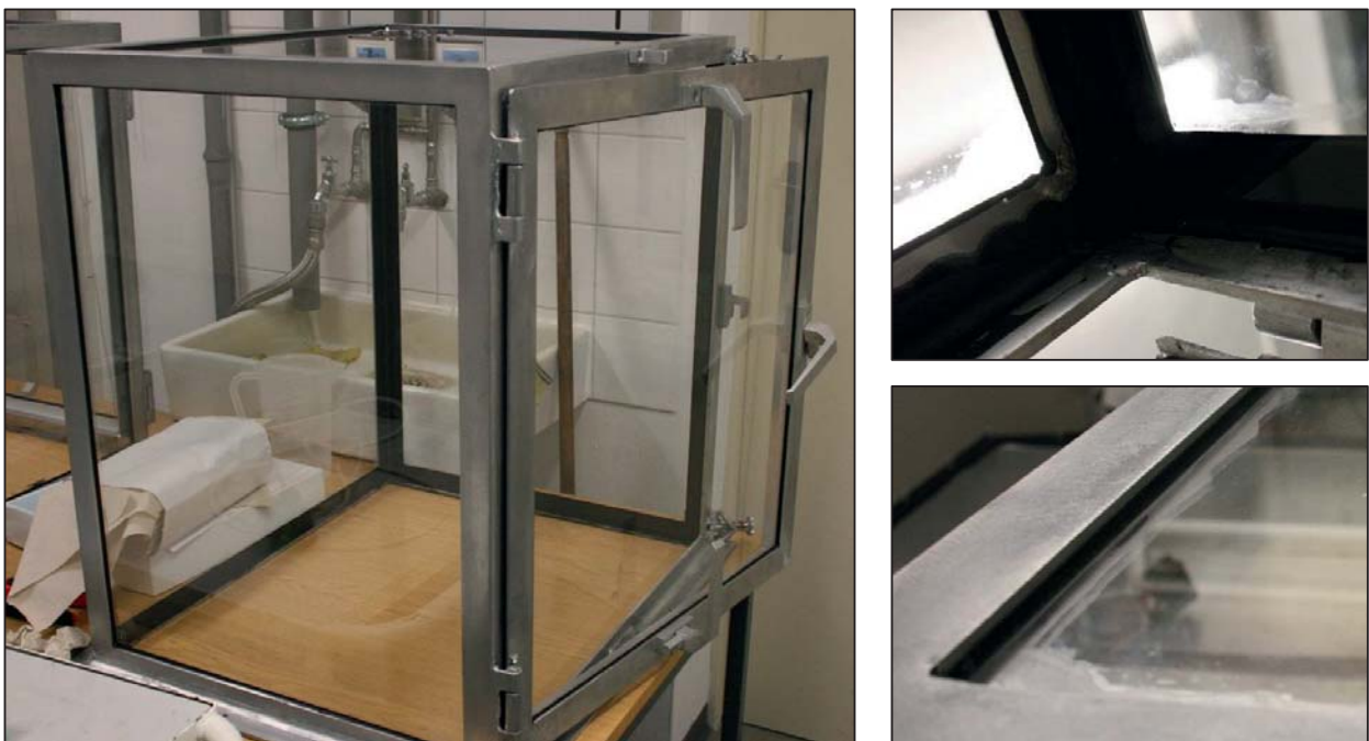
Fig. 2 Glass hood (without Biobox base; left), connection of glass panes to metal frame, interior view (top right), exterior view (down right)
