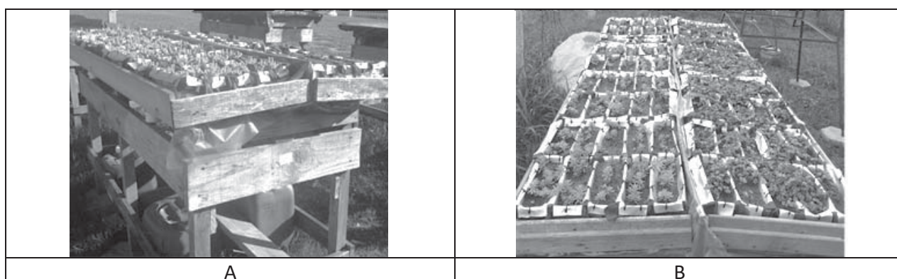
Figure 3: (A) General structure of the benches with green roof at the top and reservoirs below. (B) Distribution of plant species, Sedum rupestre on the left and Callisia repens on the right
