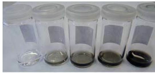
Figure 6.19.: Supernatants with increasing milling times (from left to right)
