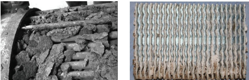
Fig. 1.1: Formation of fouling deposits inside a shell and tube heat exchanger (left) [109]; particulate fouling in a compact heat exchanger for automotive applications (right). Printed by permission from the ICTV, TU Braunschweig.
