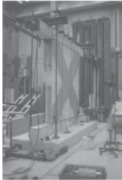
Figure 4.13: Experimental tests on masonry wall reinforced with glass fibre in the laboratory of the “Institute for Massivbau”
