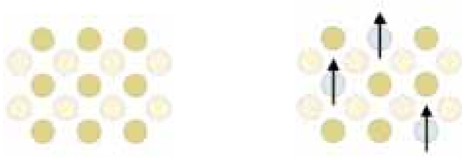
Figure 2.1: A nonmagnetic polar semiconductor (left) can be converted to a DMS (right) after diluted incorporation of magnetic ions (i.e., ions bearing a net magnetic moment) in the host lattice.
